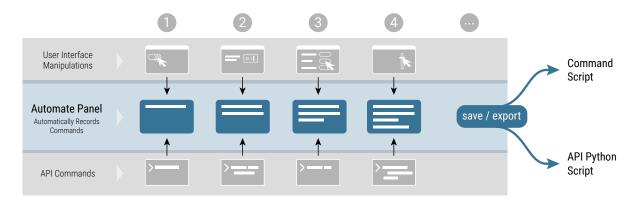
**Automate**: Skydel was built around the Command Design Pattern, which means that all actions (either from GUI or Remote control) are sent to the Engine using Commands. The commands are processed by the engine exactly the same way whether they come from the GUI or remote program. If your simulation is working via GUI, it will work exactly the same via the API.
