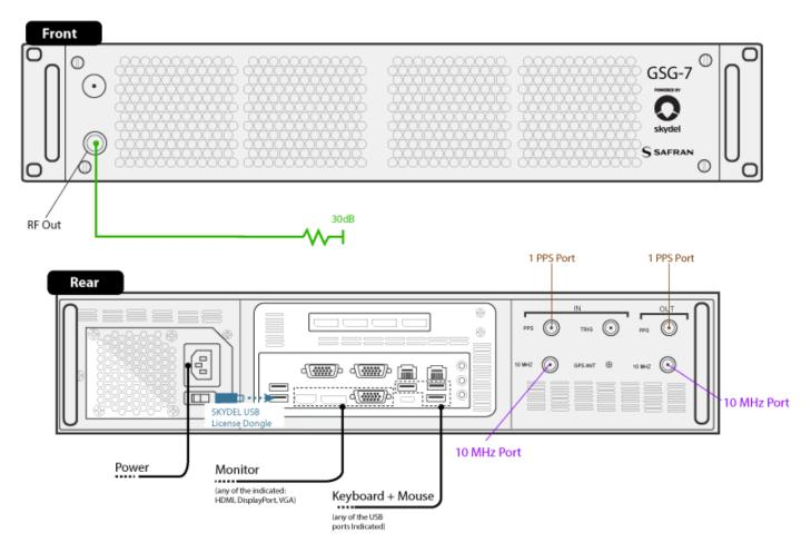
Right: The GSG-7 is equipped with an internal combiner that combines GNSS signals and bands into a single RF output.
