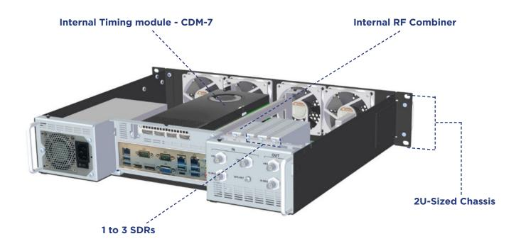
The GSG-7 has been purpose-built to provide exceptional signal quality and performance, all the while taking advantage of the latest commercial-off-the-shelf (COTS) hardware.
