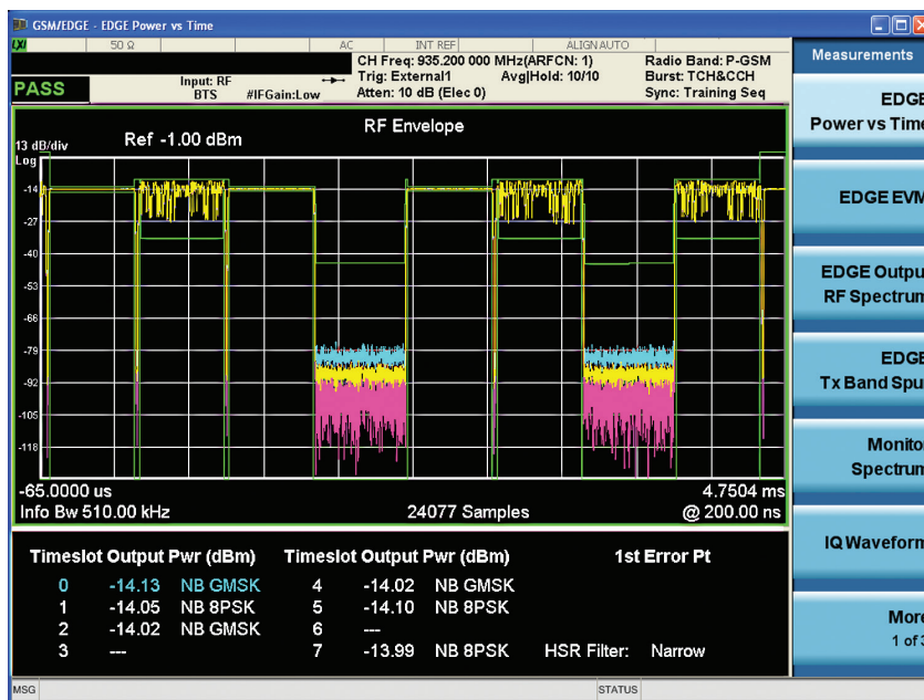
Figure 1. Multi-slot power vs. time on mixed modulation types of GSM and EDGE burst.
