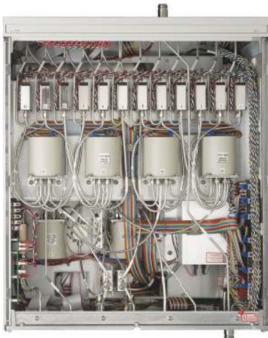
Switch matrices use high performance multi-port switches to route multiple input signals to multiple output signals simultaneously.
