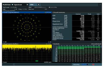
DVB-S2X signals use different modulation schemes for the payload and the header sections of the frame. The different types of modulation can be analyzed using the R&S\*FSW-K70M and R&S\*FSW-K70 options. The screenshot above shows a DVB-S2X signal using 64APSK for the payload and QPSK for the pilot channels.
