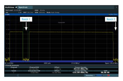
Noise power ratio measurement with the R&S\*FSW-K19 option.
