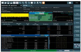
The R&S®FSW-K106 NB-IoT measurement application.
