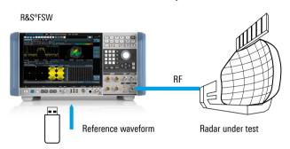
The analyzer shows trends and performs statistical analyses on all pulse, chirp and hop parameters. Trend analysis allows you to quickly identify the effects of supply voltages (or their frequencies, such as 50 Hz or 400 Hz) and to rapidly verify frequency hopping patterns and changes in the pulse repetition interval.
