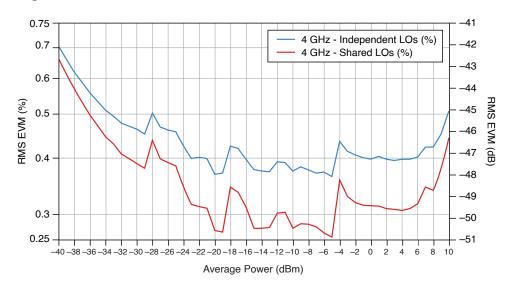
Conditions: RF output loopback to RF input; Reference/power level: average power +PAPR; Waveform bandwidth: 100 MHz; Subcarrier spacing: 30 kHz, uplink, 256 QAM; Offset Mode: Enabled; Reference Level Headroom: Default (1 dB); Measurement length: 3 slots
