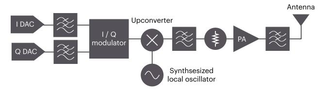
Figure 1. Diagram of a typical RF signal path, including a power amplifier
