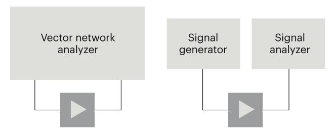
Figure 2. Traditional PA test requires a VNA for network analysis and VSA for ACPR, noise power ratio, and EVM
