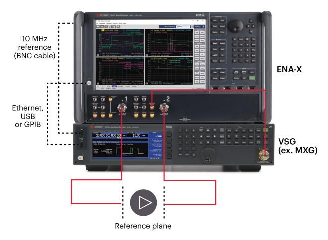
Figure 4. VNA method set-up using the ENA-X network analyzer's upconverter path with the MXG
