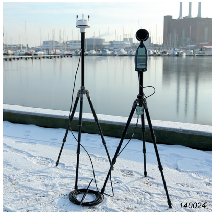
Fig. 14 Hand-held analyzer measuring outdoor noise using a weather station kit
