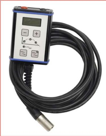
Many times, you place the test equipment on the ground while the cables are connected high up on a circuit breaker. In these situations, it can save a lot of time using a remote control during the test. The remote control has most of the functionality in the MJÖLNER 200 such as starting and stopping, setting the test current and read out the test values.
