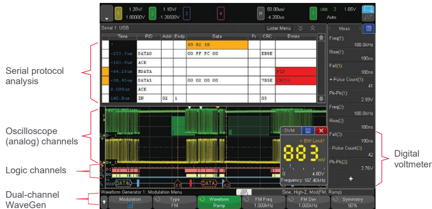
Figure 17. The 4000 X-Series provides the capabilities of five instruments seamlessly integrated into one.
