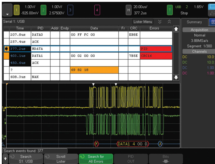
Figure 21. USB 2.0 trigger, decode and "lister" display.
