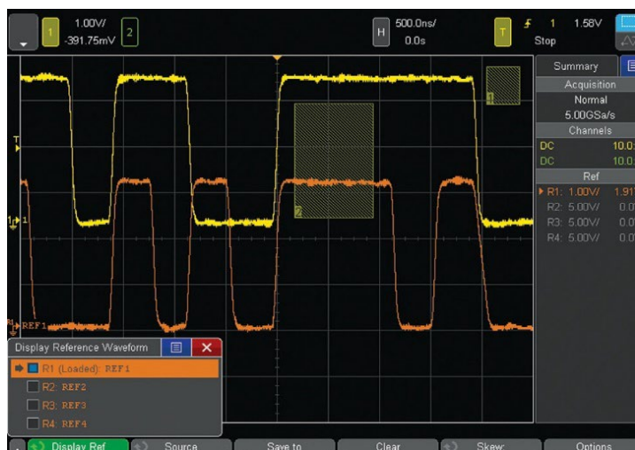
Figure 33. Store and recall up to four reference waveforms.
