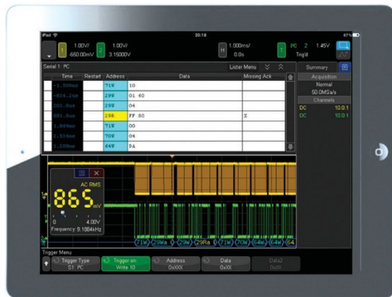
Figure 37. Tablet virtual front panel control.
