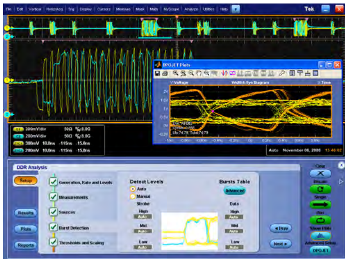
DDR Memory Bus Analysis (Option DDRA) – Automatically identify DDR1, LPDDR1, LPDDR2, DDR2, DDR3, and GDDR3 Reads and Writes and makes JEDEC conformance measurements with pass/fail results on all edges in every Read and Write burst. DDRA provides capabilities for measurements of clock, address, and control signals. In addition to enabling conformance testing DDRA with DPOJET is the fastest way to debug complex memory signaling issues. DDRA can also use the Command/Address lines to trigger on specific read/write states when running on the MSO7000 Series Mixed Signal Oscilloscope, which offers 16 channels of digital logic probing.
