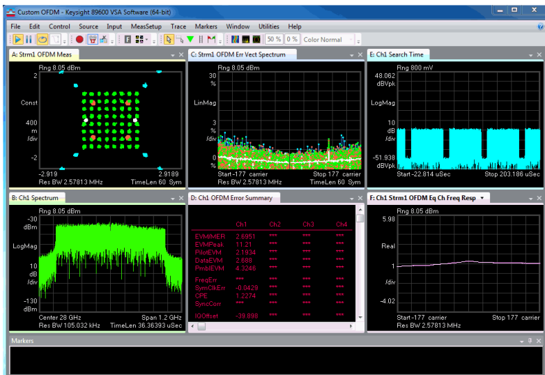
Figure 21. This display from the 89600 VSA software provides multiple views of the demodulated OFDM signal, measured with a 63 GHz Infiniium oscilloscope.
