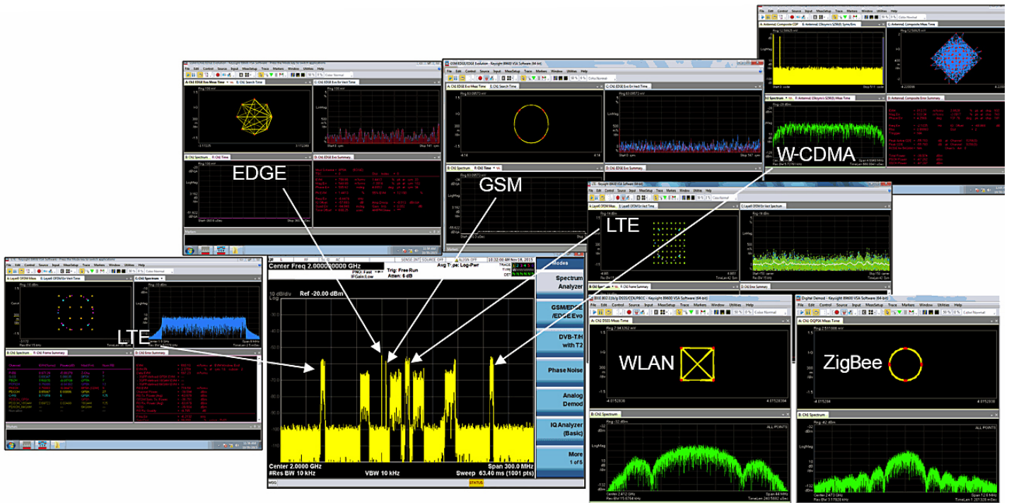
Figure 18. Demodulation of the legacy 3G, 4G, and PAN waveforms using the 89600 VSA software
