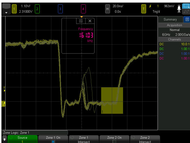
Figure 12. Hardware zone triggers immediately.
