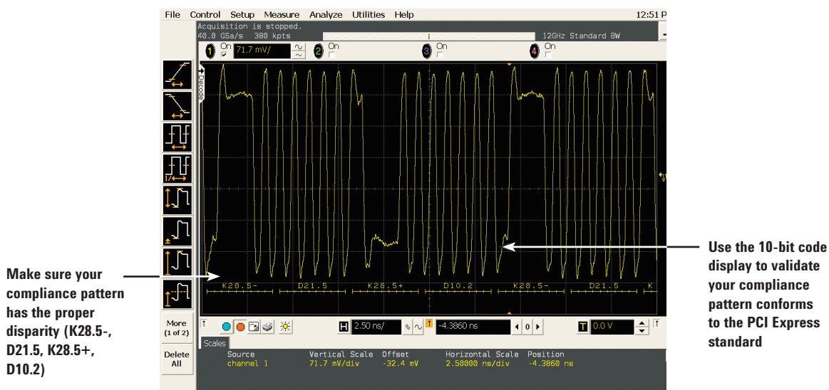
Figure 11. The 8b/10b decoded symbol information is shown below the appropriate portion of a PCI Express signal using the E2688A software.
