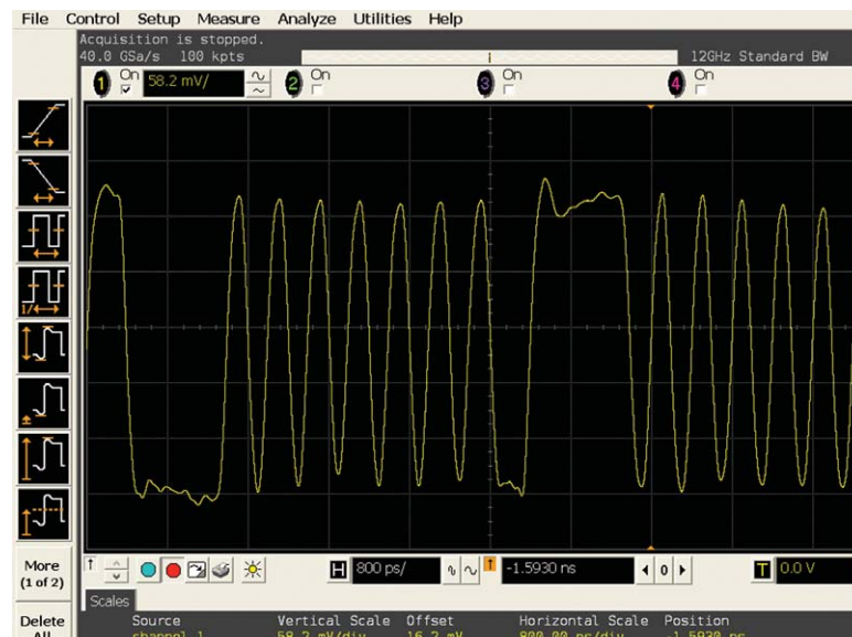
PCI Express 2.0 supports data rates up to 5.0 GT/s as shown above (-3.5 dB de-empasis)
