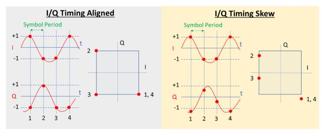
Figure 9. Example of I/Q timing skew
