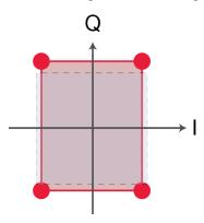
Figure 8. I/Q gain imbalance in a constellation diagram
