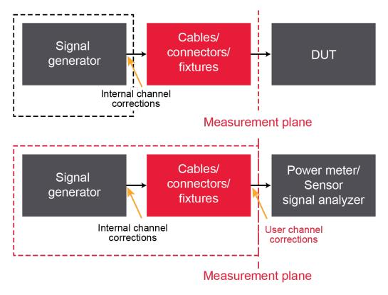
Figure 4. Move the measurement plane from the signal generator's output to the DUT's input
