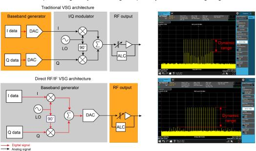
Figure 12. Comparison of analog and digital up-conversion methods
