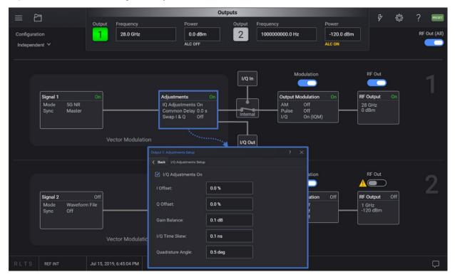
Figure 11. Baseband I/Q adjustments setup
