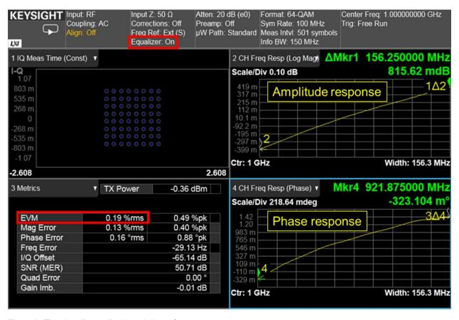
Figure 2. The signal's amplitude and phase frequency responses
