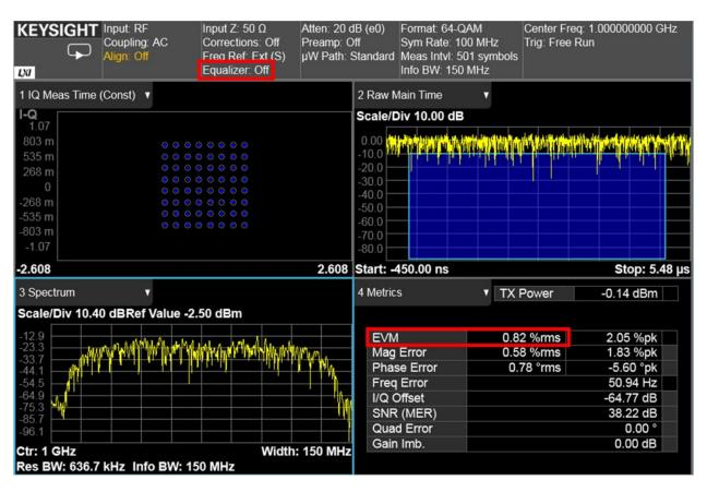
Figure 3. Signal generator with internal channel correction "on"
