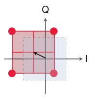
Figure 7. I/Q origin offset in a constellation diagram
