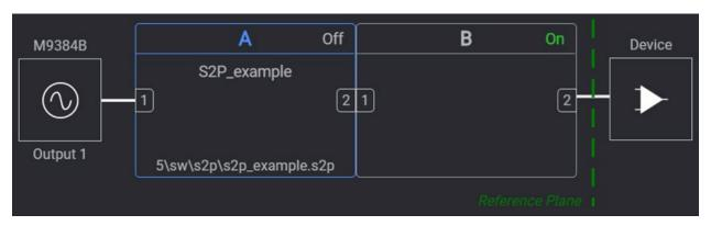
Figure 5. Cascade the channel corrections from the A and B blocks
