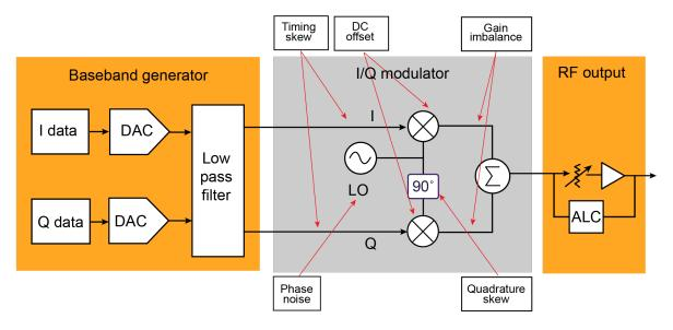
Figure 6. A block diagram of an I/Q modulator and possible errors
