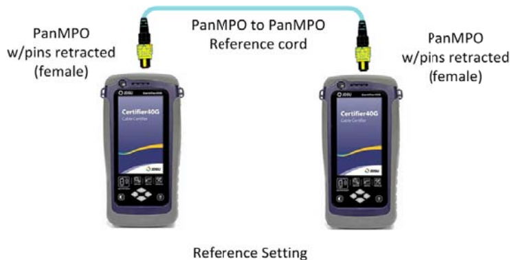
Figure 1. One-Jumper Reference Setup when Testing Method A or Method B Female Based Horizontal Cabling Infrastructure
