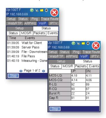
**VoIP Expert** – Generates industry standard wave files to verify MOS and R-Factor values of upstream and downstream paths and includes QoS measurements such as packet litter, packet loss, and delay. Compatible with all VeEX testers including VX1000 VoIP server software.
