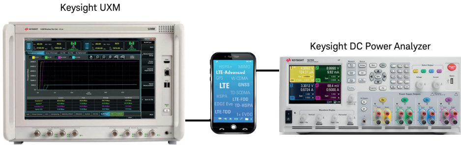
Figure 16. Battery drain test solution example includes UXM and N6705B power analyzer
