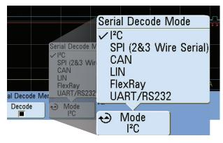
Real-time hardware-based serial decode for I<sup>2</sup>C, SPI, CAN, LIN, RS-232/UART, and I<sup>2</sup>S.
