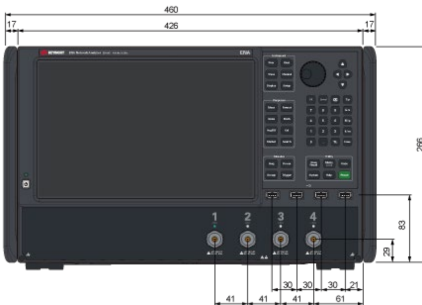
Dimensions (front view, E5080B with option 4M0/4N0/4M2/4N2 (2.4 mm), in millimeters)
