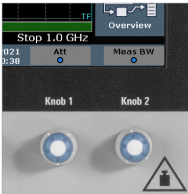
Two rotary knobs with user-assignable functions.
