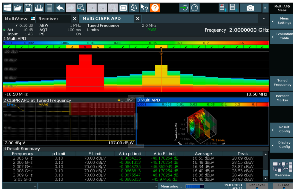
APD multichannel measurement display.
