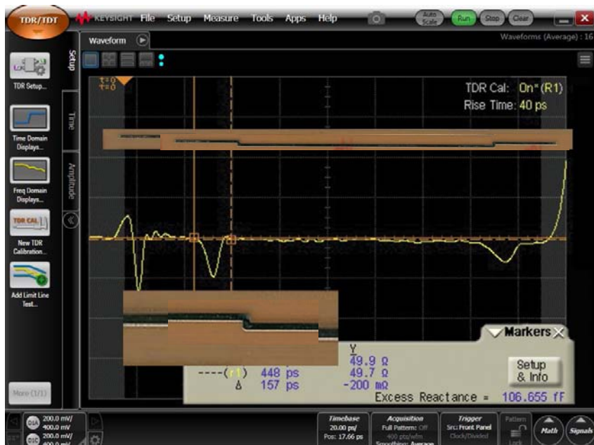
Figure 18. Using markers to extract the excess capacitance of two corners.
