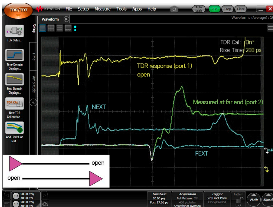
Figure 42. Measured cross talk in quiet line with worst case termination.
