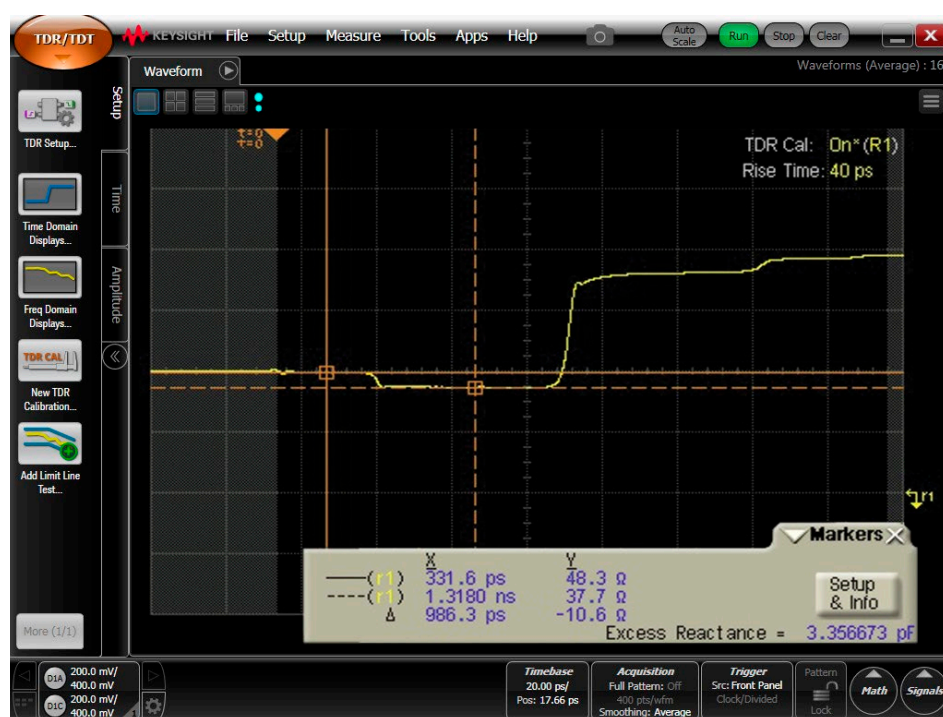
Figure 2. Using markers to measure the characteristic impedance of a transmission line.
