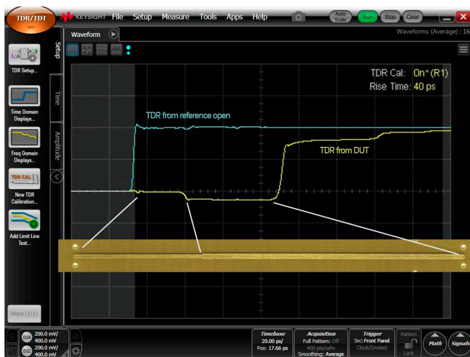
Figure 1. Measured TDR response from a microstrip transmission line. Blue trace is the reflection from the end of the cable; yellow trace is the reflected signal from the DUT.
