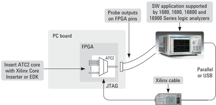
Figure 2. Create a timesaving FPGA measurement system. Insert an ATC2 (Agilent Trace Core) core into your FPGA design. With the application running on your logic analyzer you control which group of internal signals to measure via JTAG.
