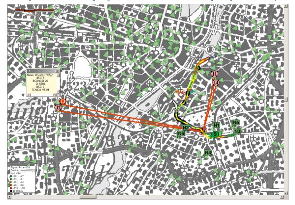
To optimize interference analysis, more than just selectable trigger thresholds (e.g. RxLevFull, RxLevSub, RxQualFull, RxQualSub, FER) are used. Some of the test mobile phones supported by R&S®ROMES4 also provide a C/I value for the traffic channels being used (TCH). Because the SIM connection only allows the test mobile phone to see the data from the allocated mobile network, and because it is not very RF-sensitive, the use of high-grade scanners is absolutely essential.
