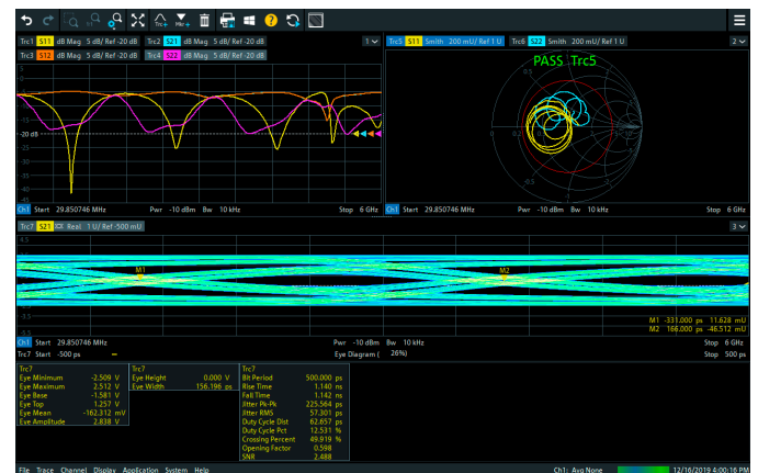
Simultaneous display of eye diagrams and measurements in the frequency and time domain
