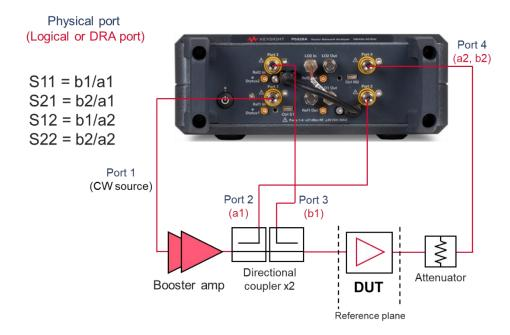
External components should be selected based on their high-power limits or frequency range specifications. Be sure that these components can handle the output power level of the booster amplifier.
