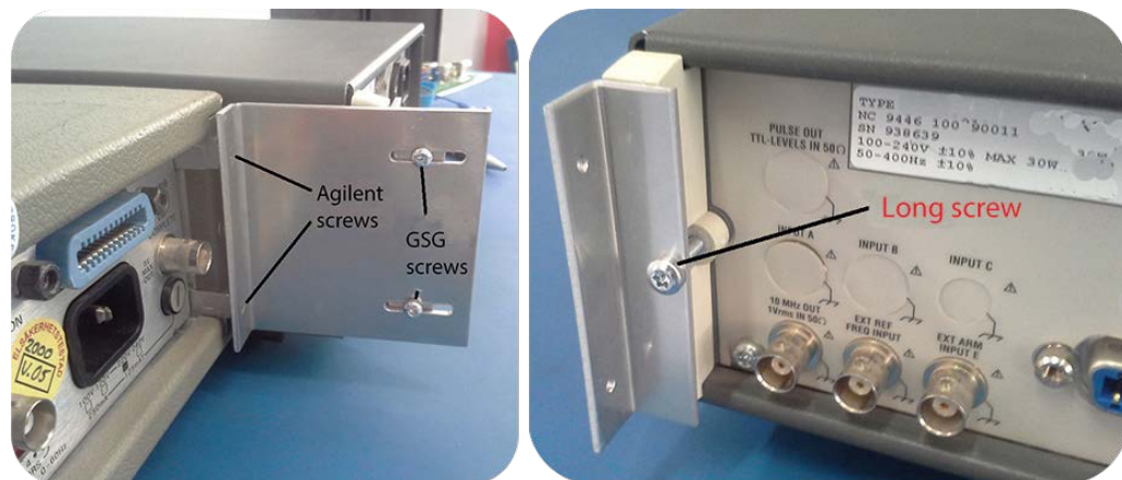
Figure 2-10: Installation of rear assembly plates
