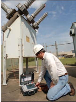
**The S1-552 Insulation Resistance Tester in use at an industrial complex substation**
