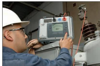
**Circuit breaker being tested with the S1-552 Insulation Resistance Tester**
