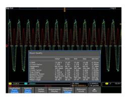
With the DPO4PWR Power Analysis Application Module installed on an MDO4000 Series oscilloscope, an embedded designer who rarely deals with power measurements can quickly get the same accurate, repeatable results as a power supply expert. A Power Analysis Application Module with an oscilloscope and differential voltage and current probes form a complete measurement system for power supply design and test.
