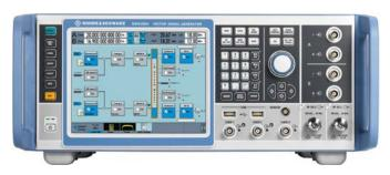
The SMW200A is the vector signal generator for the most demanding 5G applications. It offers flexibility, performance, and intuitive operation for generating complex, digitally-modulated signals of high quality for 5G LTE Advanced to 2G applications.
