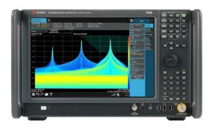
The N9040B Signal analyser offers real-time spectrum performance analysis up to 1GHz for deeper views of complex and challenging 5G signals. Clean spectral purity with leading phase noise measurements. Extendable frequency range to 110GHz with external smart mixers.
