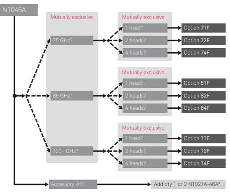
\* Each N1027A-46A accessory kit supports one differential channels (two heads).
