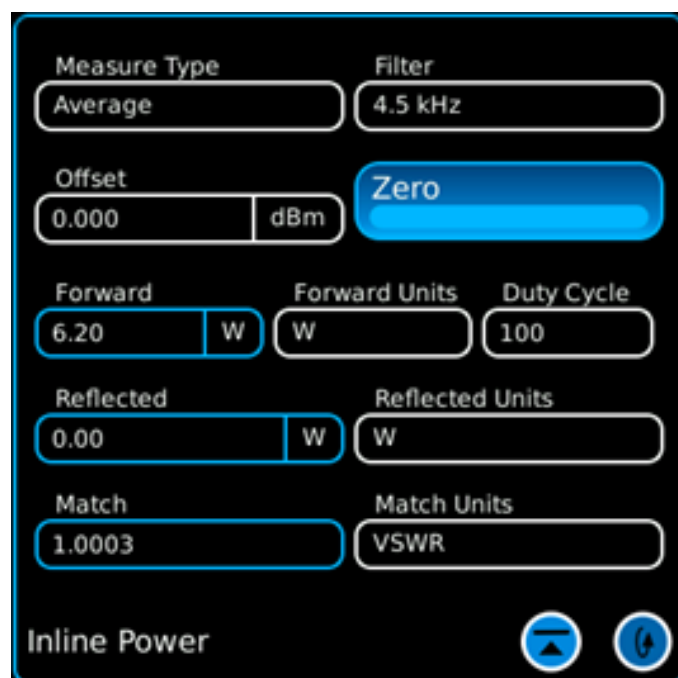
In-Line Power Meter Tile
