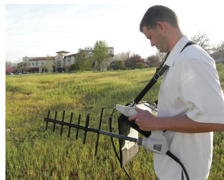
Figure 18. The Hand Held Interference Hunter in-use
