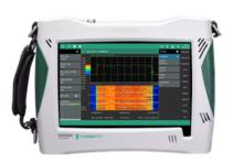
The portable spectrum analyzer MS2090A has been designed with at least one major emerging wireless application in mind: testing the various signal components of the next version of cellular radio technology - 5G New Radio (5G NR) wireless systems.
