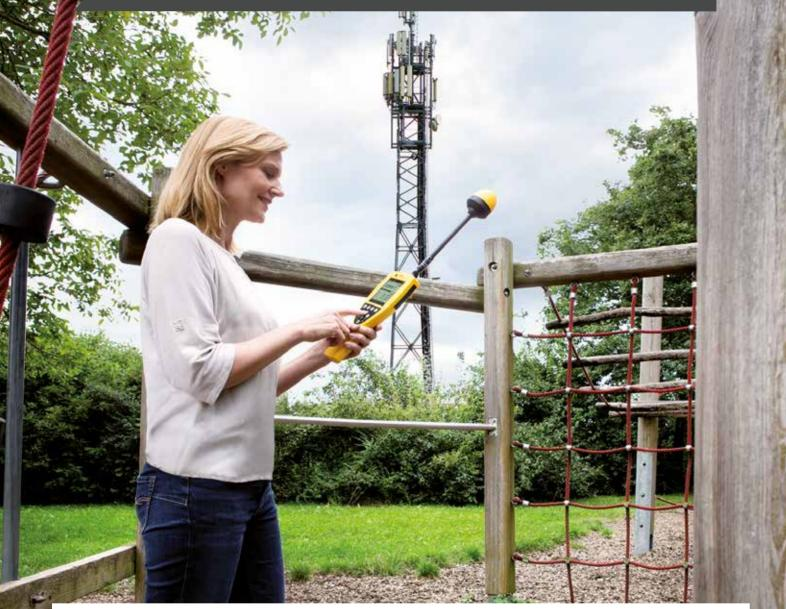
The places where field strengths need to be measured are often not the most convenient. The Narda Broadband Field Meters in the NBM-500 series are therefore designed to be used anywhere. The casings are impact resistant, the probes are robust. The monochrome displays – backlit LCDs – can be read in darkness and in bright sunlight. Even under difficult working conditions, you will immediately get reliable results. Narda offers two device types with a wide range of probes,
