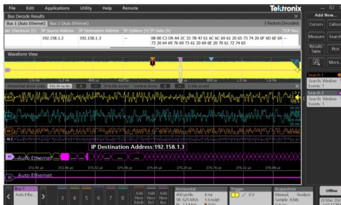
100BASE-T1 Protocol decode on PC based TekScope Application
