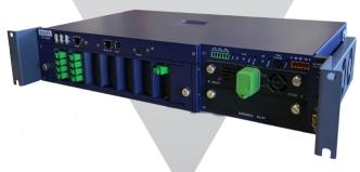
The OTU-8000 Optical Test Unit lies at the core of the Viavi Solutions® optical network monitoring system (ONMSi). Combining optical time-domain reflectometry (OTDR) and optical-switch technology, a single OTU-8000 unit can test hundreds of fiber links. When a fiber fault occurs, the ONMSi reports the GPS location of the fault within minutes.
