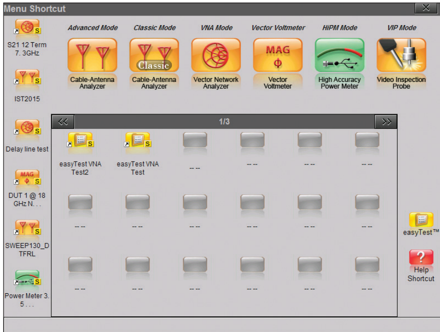
Main menu screen provides one touch mode selection and access to setup shortcuts
