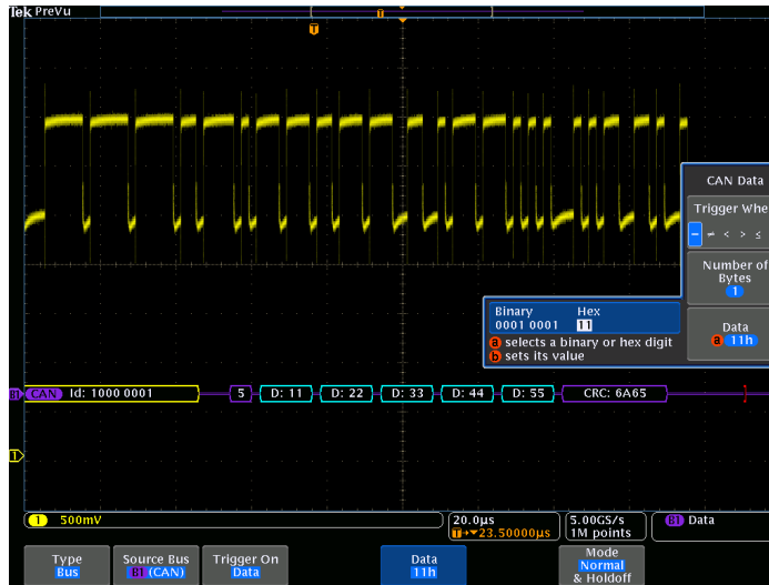
Figure 16: Triggering on a specific data value on the CAN bus.
