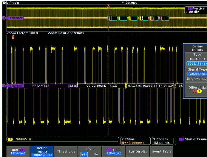
Figure 35: Color-coded DPO4ENET display of 100BASE-TX.
