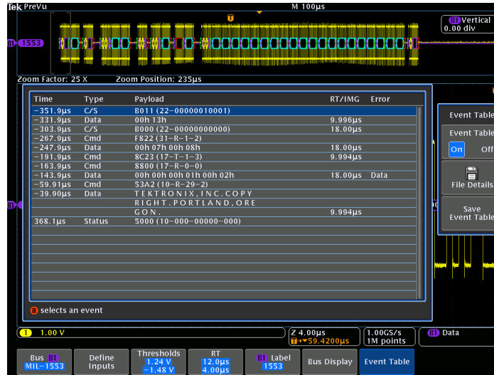
Figure 28: Event table for MIL-STD-1553 bus with all captured packets time stamped and in a tabular view.
