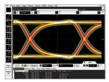
Figure 2. Direct signal connect to Infiniium scope
