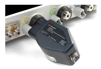
The Keysight N7004A optical-to-electrical converter is a high-sensitivity photodetector module designed for direct optical-to-electrical conversion of optical telecom or data com signals into an Infiniium real-time oscilloscope with AutoProbe II interface.
