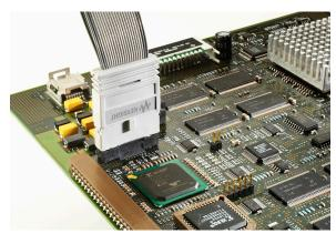
E5346A 34-channel Mictor connector probe
