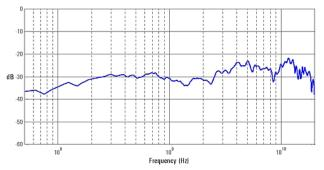
Common mode rejection ratio of 1169B
