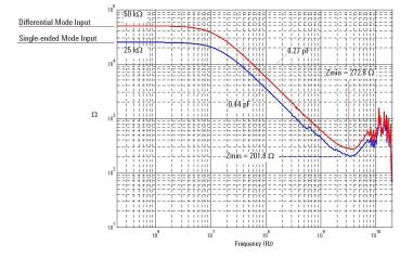
Probe input impedance versus frequency
