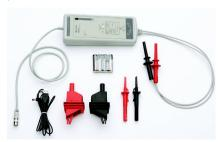
N2891A 70 MHz high voltage differential probe
