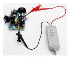
N2790A measuring a power supply signal
