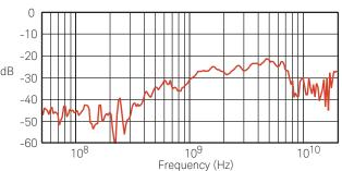
Common mode rejection versus frequency
