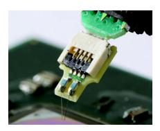
N2887A InfiniiMax Soft touch Pro Probe Adapter adapts from the Keysight Pro Series (36 ch) Soft touch connectorless logic analyzer foot print to the Keysight InfiniiMax I and II Series probe amplifier input connectors.
