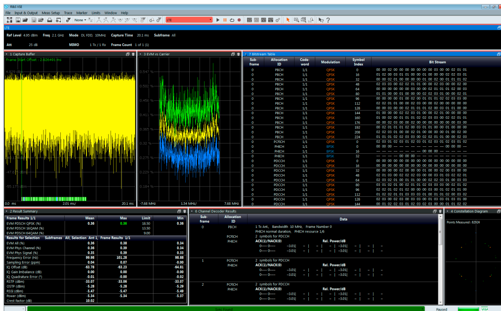
An LTE downlink signal with modulation results and in-band measurement results such as bitstreams and information gained by control channel decoding.
