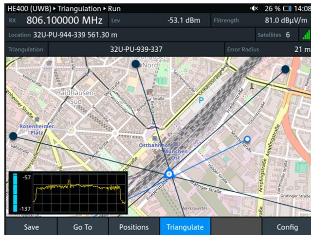
Mapping tools such as triangulation or level mapping with an integrated spectrum view
