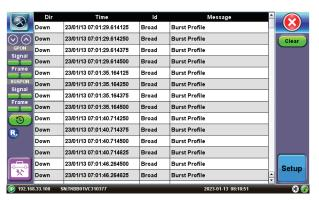
The PLOAM messaging can also be used to determine OLT commands to ONT including ONT disconnect commands.
