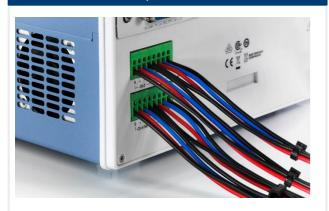
Connections for all channels – including sense – are also provided on the rear panel
