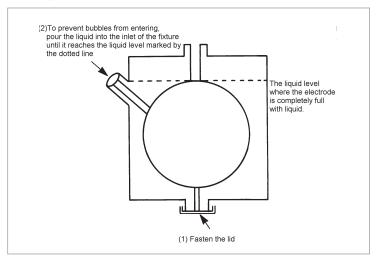
Pouring the liquid into the fixture
