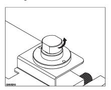
Remove the cap of the fixture
