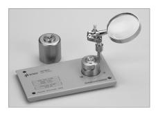
Terminal Connector: 7 mm DUT Connection: 2-Terminal Electrical Length: 27.3 mm
