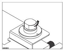
Remove the cap of the fixture
