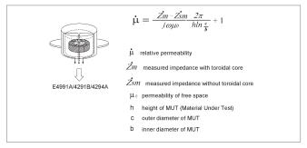
Permeability measurement method of 16454A
