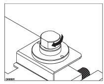
Replace the cap by screwing tightly
