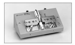
Terminal Connector: 4-Terminal Pair, BNC
