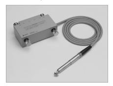
Terminal Connector: 4-Terminal Pair, BNC
