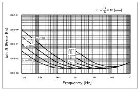
Typical Loss Tangent (tan  $\delta$ ) Measurement Accuracy ( $\otimes$  h\* ln c/b = 10)
