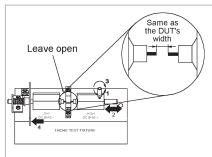
Put the DUT where it is touched by the end of the low electrode.
