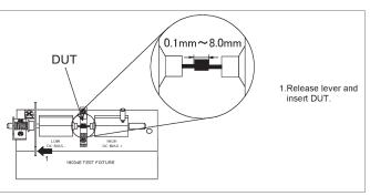
Inserting a DUT
