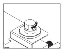
Replace the cap by screwing tightly
