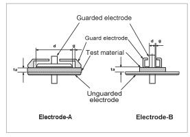
Electrodes for contacting electrode method (Rigid Metal
