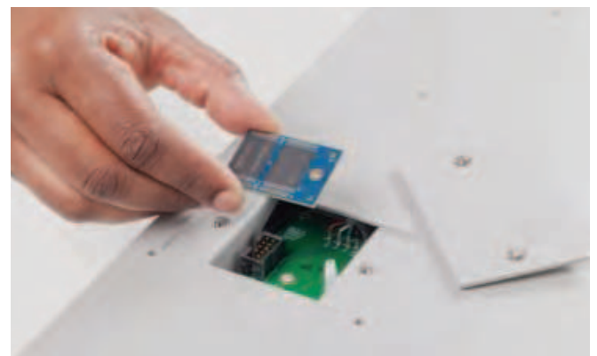
Figure 8. Installing the N7908A BBR hardware option on an APS power supply
