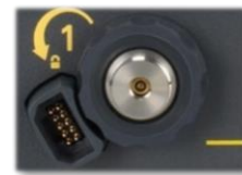
Ruggedized 3.5 mm Male Bulkhead Connector with AutoProbe II Interface
