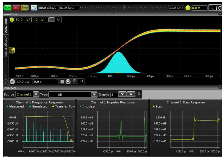
InfiniiSim renders the waveform through hardware acceleration
