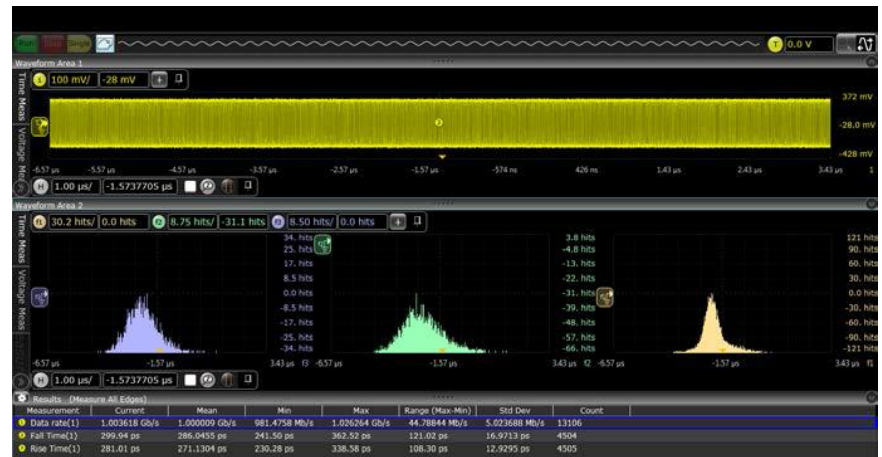
With its flat frequency response and low noise, the UXR-Series can accurately measure jitter components such as ISI.
