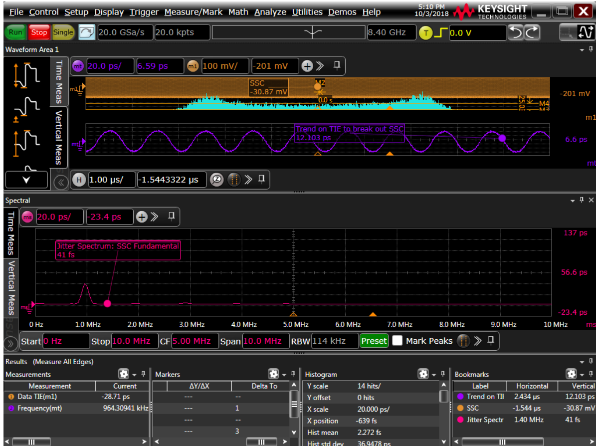
Figure 5. Results of the measurement setup wizard show the jitter histogram, trend, and spectrum.
