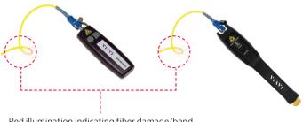
Red illumination indicating fiber damage/bend
