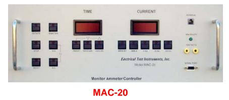
**INITIATE key:** This key is used to turn ON the output of the test set. The LED in the key indicates that the MAC-20 is attempting to turn the output ON. In MOMENTARY mode, the key must be held to keep output current on. In MAINTAIN mode, once current is detected, the output will stay on until the breaker trips, or the STOP or RESET button are pressed.
