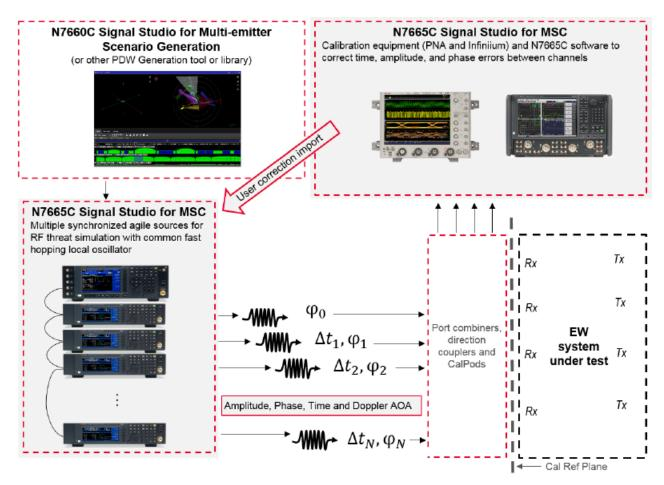
**Signal Studio for Multi-Source Calibration (MSC)** is designed to automate alignment of AoA parameters (Amplitude, phase and/or Time) for a set of UXGs in a system with a calibration reference plane at the connection ports of the SUT.
